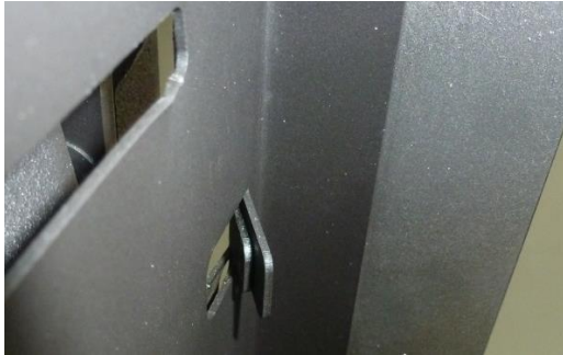
Figure No.13 - Close up of the bent tab
