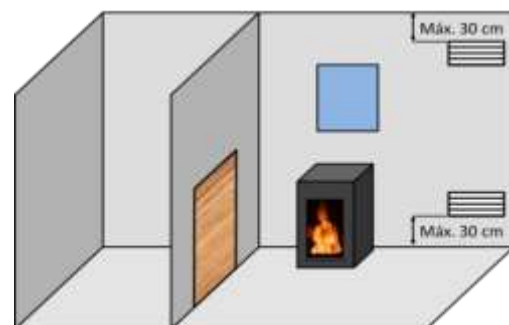
Figure No.3 - Guideline indications for ventilation grilles
