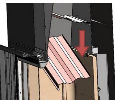
Figure No.25 - Dismantling the lower Inca deflector
